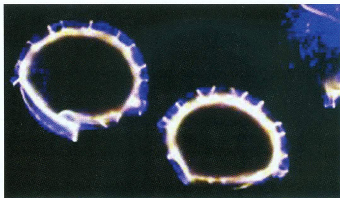
Figure 6 Confocal microscope picture of empty 25 micron (25 \mu\text{m} ) diameter pollen shells. Reproduced with the permission of Sporomex Ltd.
